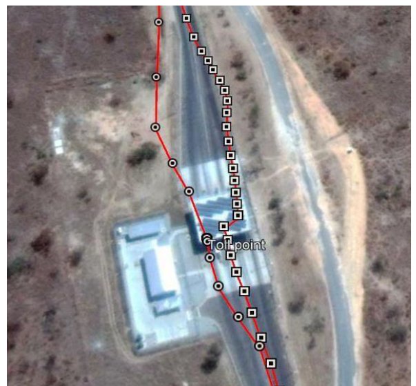
Figure 1: Diagram showing vehicle movement tollpoint tracking at Gweru-Kwekwe tollgate to-and-from route.
