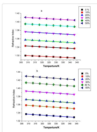
Figure 5: The dependence of refractive index of sugar solution on temperature at different concentrations using **a**. Red diode laser (650 nm) and **b**. Green Diode laser (532 nm).
