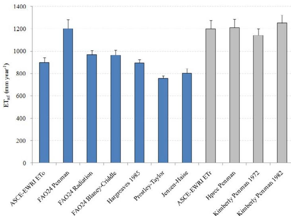
Figure 5: Comparison of annual reference evapotranspiration values ( $ET_{ref}$ ) for all methods. The dark color bars indicate the grass reference based methods and the light color bars indicate the alfalfa reference based methods. The error bars indicate the standard deviation among the 18 years.
