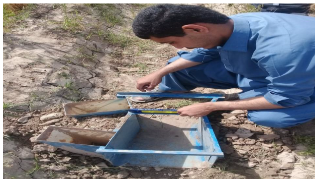
Figure 4: Installation of cut throat flume at the channel for flow measurement.
