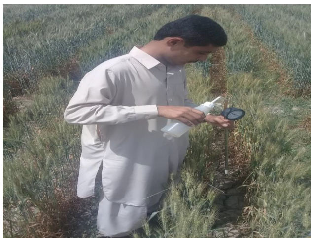
Figure 5: Installation of tensiometer at the field.
