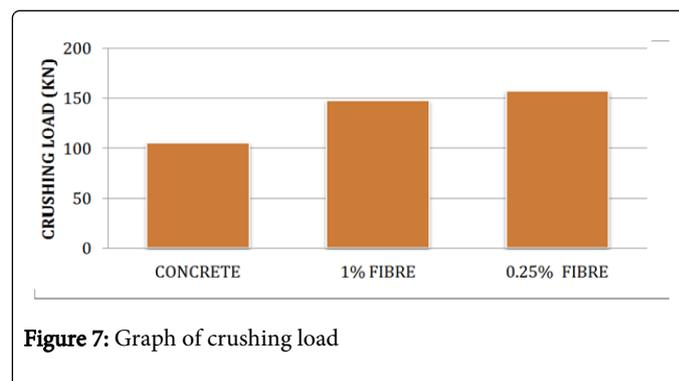
Figure 7: Graph of crushing load
