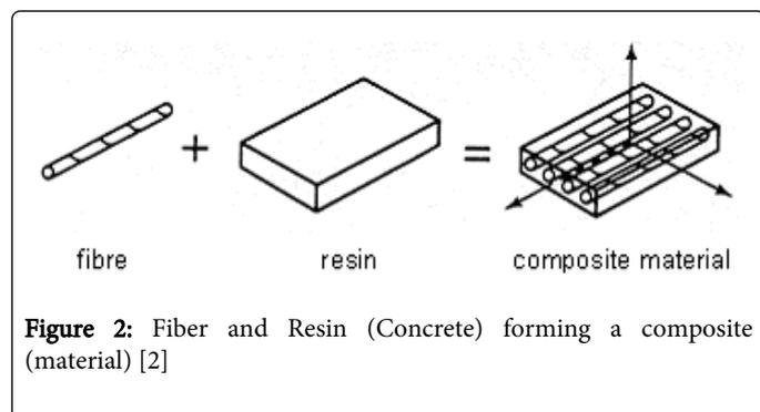
Figure 2: Fiber and Resin (Concrete) forming a composite material [2]
