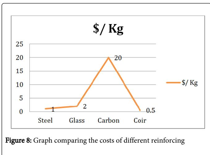
Figure 8: Graph comparing the costs of different reinforcing
