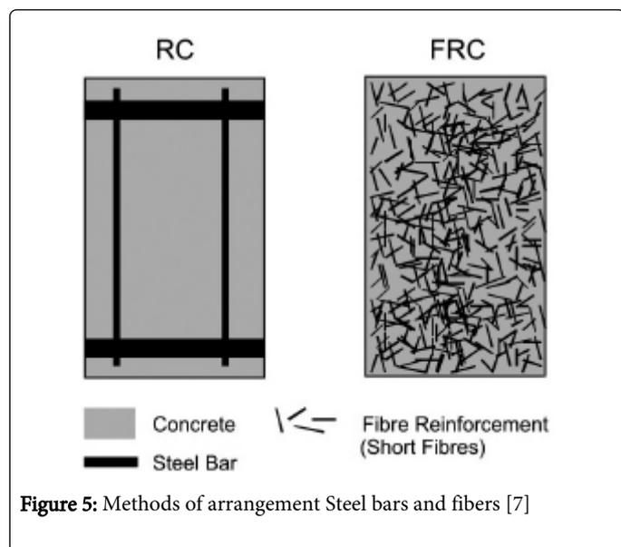
Figure 5: Methods of arrangement Steel bars and fibers [7]
