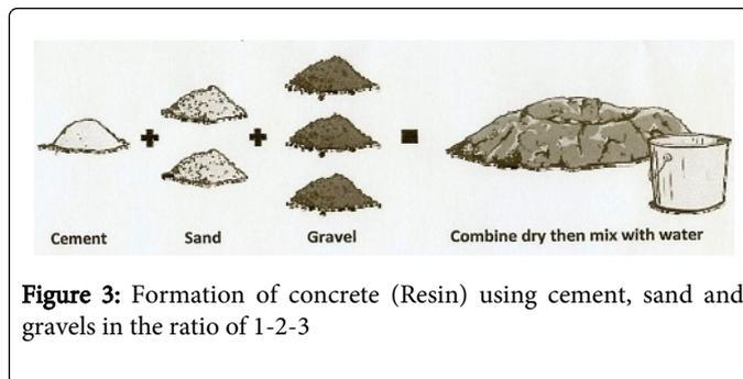
Figure 3: Formation of concrete (Resin) using cement, sand and gravels in the ratio of 1-2-3
