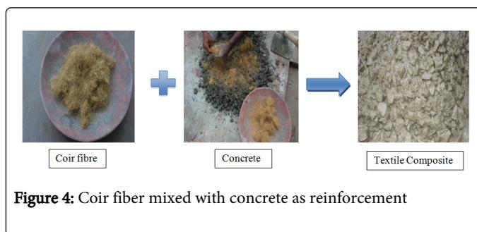
Figure 4: Coir fiber mixed with concrete as reinforcement
