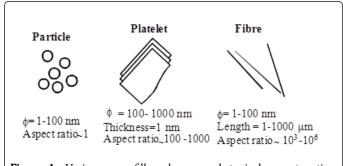
**Figure 1:** Various nanofiller shapes and typical aspect ratios. Reproduced with permission from Pillai and Ray [80].
