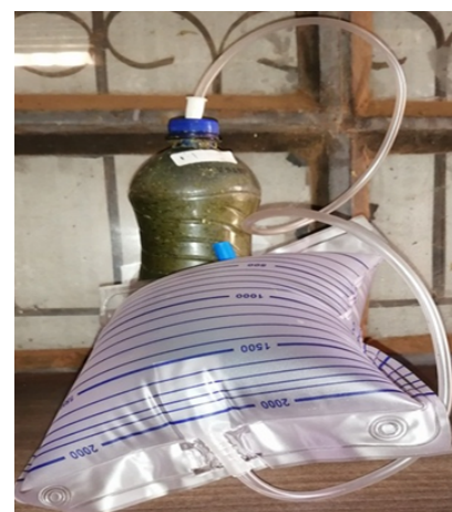
Figure 2. Biogas production and storage set up.
