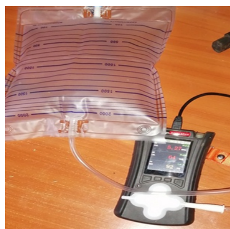
Figure 3. Biogas composition measurement using GP180.
