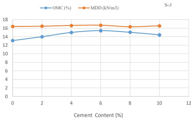
**Figure 3.** Variation of maximum dry density and optimum moisture content with percentage cement content for soil sample S-3.
