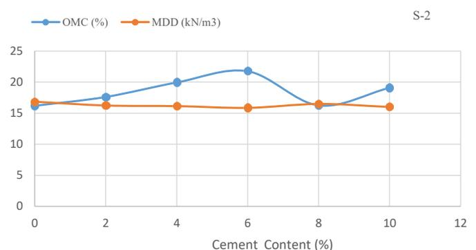
Figure 2. Variation of maximum dry density and optimum moisture content with percentage cement content for soil sample S-2.
