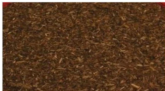
Figure 3. Date palm leaves cut into small size and pre-carbonized in a vacuum chamber at 280^\circ\text{C} .
