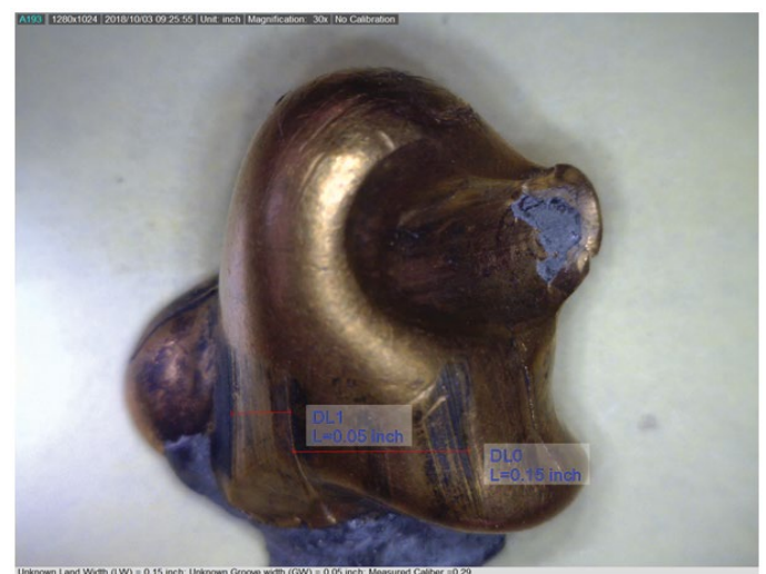
Figure 6. Sample bullet three of a highly deformed jacketed bullet fired from a foreign made pistol (3.0) with the digitally measured land width = 0.15 (dlo, right), the digitally measured groove width = 0.05 inch (dl1, left), and the known diameter = .30 inch from the fired casing.
