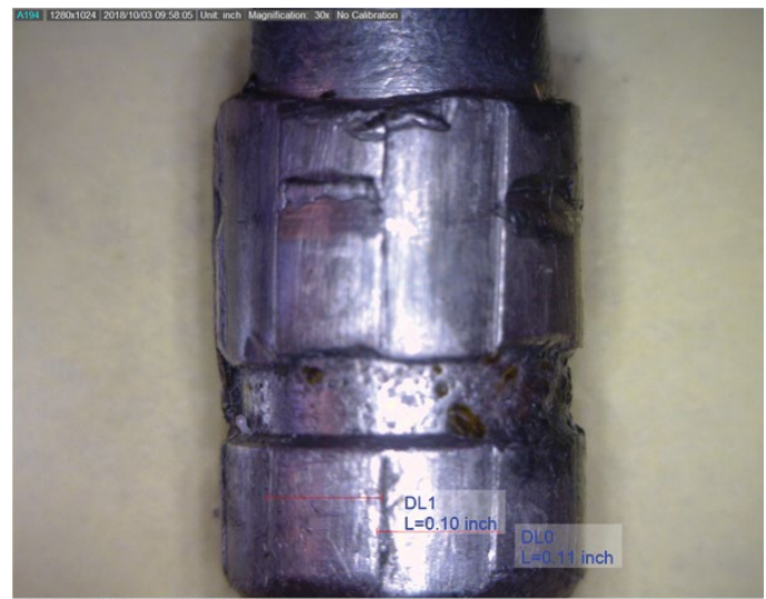
Figure 5. Control sample two (intact) by a .38 with the digitally measured land width = 0.10 inch (dl1, left) and the digitally measured groove width = 0.11 inch (dlo, right).
