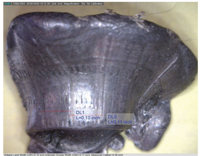
Figure 4. Sample bullet two of a highly deformed lead bullet fired by a revolver (.38) with the digitally measured land width = 0.10 inch (dl1, left) and the digitally measured groove width = 0.11 inch (dlo, right).
