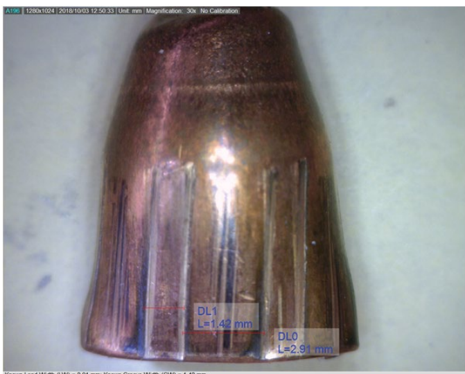
Figure 3. Control sample one fired by a pistol (9 mm) with the digitally measured land width = 2.91 mm (dlo, right) and the digitally measured groove width = 1.42 mm (dl1, left).
