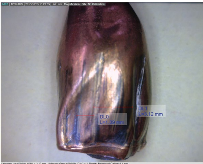
Figure 2. Sample bullet one of a highly deformed jacketed bullet fired by a pistol (9 mm) with the digitally measured land width = 3.12 mm (dl1, right) and the digitally measured groove width = 1.39 mm (dlo, left).
