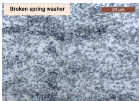
Figure 4a: 3% Nital Etched microstructure of failed twisted Sample 1.
