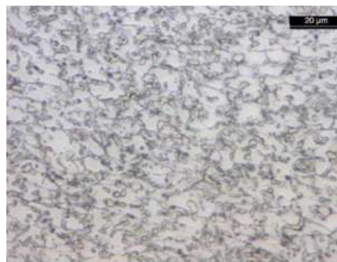
Figure 5b: 3% Nital Etched microstructure of flat failed samples before heat treatment.
