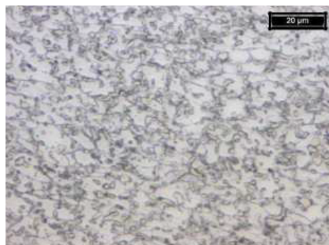
Figure 5c: 3% Nital Etched microstructure of flat failed samples after heat treatment.
