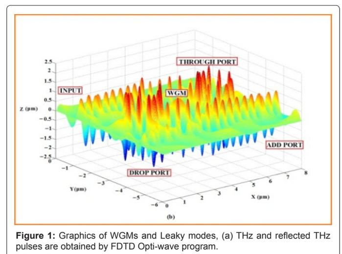
Figure 1: Graphics of WGMs and Leaky modes, (a) THz and reflected THz pulses are obtained by FDTD Opti-wave program.
