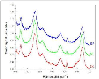
**Figure 4:** Raman spectra of the EP, ST and ZK groups. The peaks identified are related to Yttria tetragonal Y-TZP polycrystalline structures ( ~260, 320, 464, and 147cm<sup>-1</sup>).
