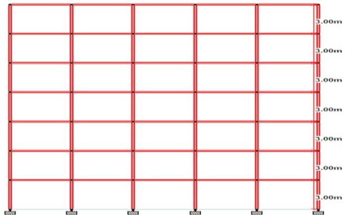
**Figure 2.** Elevation of the 7 storeyed RCC structure.
