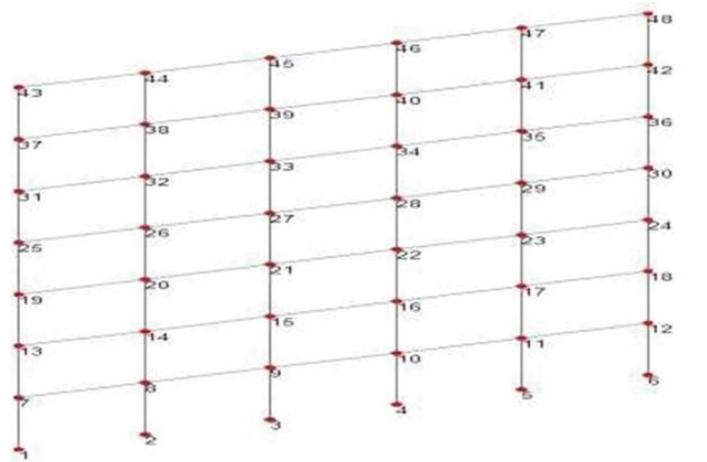
**Figure 4.** STAAD Pro model showing blast forces acting on the nodes.
