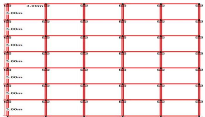
Figure 1. Plan of the 7 storied RCC structure.
