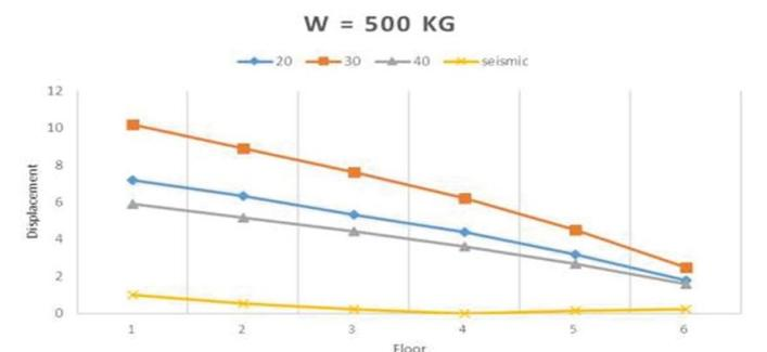
**Figure 5.** Displacement in mm at each floor for charge 500 kg.
