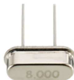
Figure 11: HS-49S Crystal Oscillator (8 MHz).
