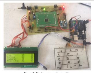
Figure 3: Display menus at transmitter.
