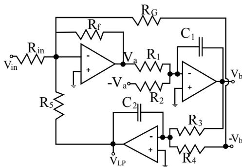
Figure 3: 2<sup>nd</sup> order Low Pass Filter applying difference approach topology.
