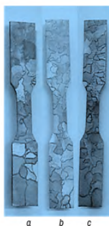
Figure 17. Macrostructure of Inconel 718 alloy:(a) without NM, (b) with TiN + NiAl, (c) with (TiN+TiCN) + NiAl. The sample diameter is 20 mm
