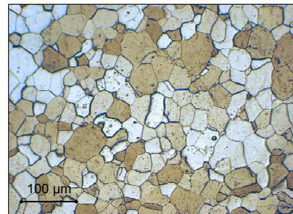
**Figure 9:** Micrograph obtained by optical microscopy, showing a fine-grated area with no twins.
