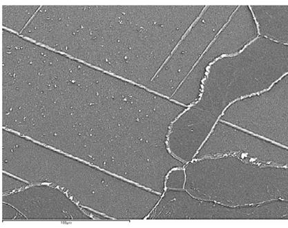
**Figure 14:** Detail, at higher magnifications of the area shown in Figure 13, showing how the iron carbides mark perfectly the grain boundaries and twin planes.
