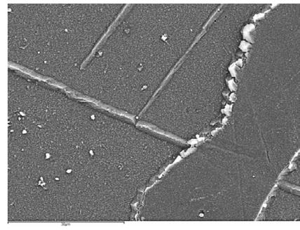
**Figure 15:** Detail, at higher magnifications in the area of Figure 14, showing the morphology of the iron carbides of twins and grain limits.
