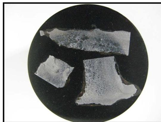
Figure 5: Macrograph of sectioned iron nail subjected to deep drawing, grinding, polishing and chemical attack with 2% Nital.
