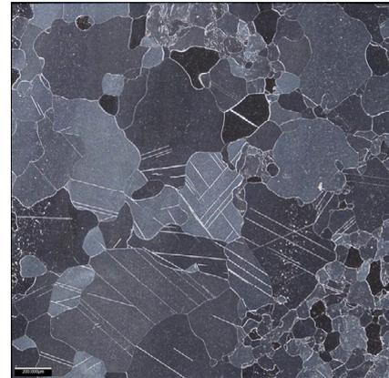
**Figure 7:** Macrograph with confocal magnifying glass that shows the existence of maclas in those grains that have grown during recrystallization.
