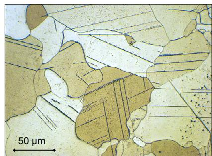
**Figure 10:** Micrograph obtained by optical microscopy, showing the twinning in grains of great growth.
