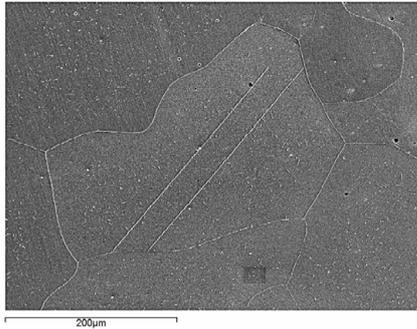
**Figure 11:** Micrograph obtained by scanning electron microscopy, showing the twins and grain limits marked with iron carbides.
