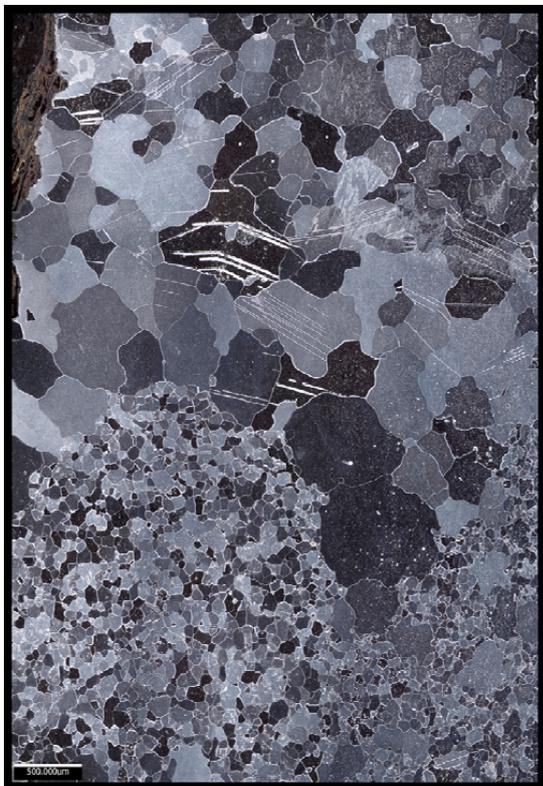
**Figure 6:** Macrograph with confocal magnifying glass showing one grain growth zone and another small grain zone. The twins are only in the grains that have grown.
