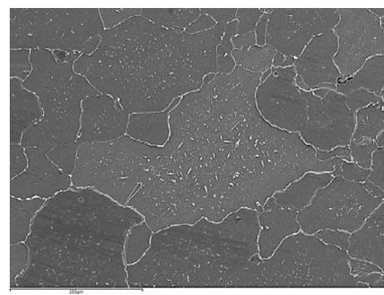
**Figure 16:** Micrograph obtained by scanning electron microscopy, showing an area of small grains. Carbides are observed at grain boundaries and in the ferritic matrix with Widmanstätten structure.
