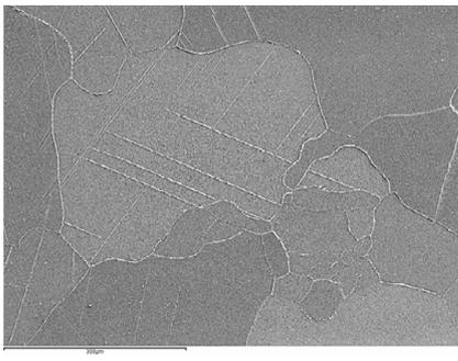
**Figure 13:** Micrograph obtained by scanning electron microscopy, showing the numerous grain twins and grain limits of the grain growth zone.
