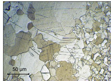
**Figure 8:** Micrograph obtained by optical microscopy where the existence of twins in the coarse grains is appreciated.
