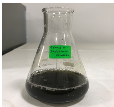
Figure 1. The cinnamon and clove mediated gold particles solution color changed to blackish brown within 48 hours of reaction with gold chloride solution.
