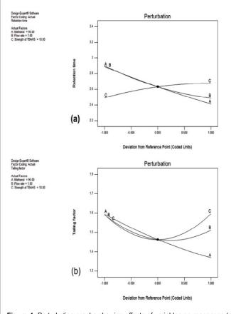
**Figure 4:** Perturbation graphs showing effects of variables on responses (a) Retention time-Y<sub>1</sub>, (b) Tailing factor-Y<sub>2</sub> [A=Methanol (%); B=Flow rate (mL/min) and C=Strength of TBAHS (mM)].
