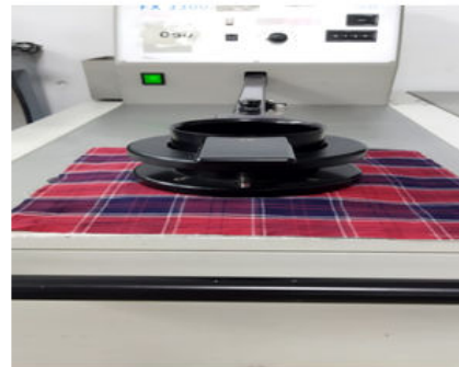
Figure 4. Air porousness transmission measurement process of fabrics.
