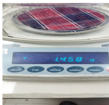
Figure 1. Weight (g/m 2 ) measurement of the fabric.
