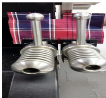
Figure 2. Tear strength measurement observed by James heal tear tester machine (Elmendorf).
