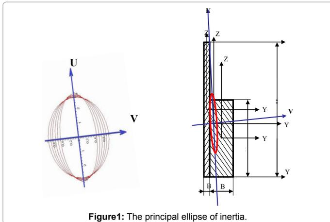
Figure 1: The principal ellipse of inertia.
