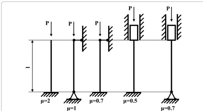
Figure 4: Shows several types of fixing rod and indicate the relevant values of the coefficient  $\mu$  - the so-called coefficient of length is given.
