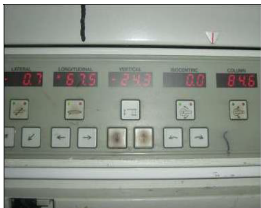
Figure 4: The digital reading as displayed on the couch control panel. Each value can be zeroed in order to assist setup, but the absolute values are captured and stored by the LANTISTM for each treatment.
