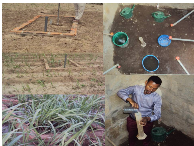
Figure 2. Partial view of lysimeter: A) Soil sampling from lysimeter, B) Sugarcane germinated in the lysimeter C) Sugarcane at tillering stage, D) Lysimeter drainage hole and E) Measuring deep percolated water from lysimeter drainage hole.
