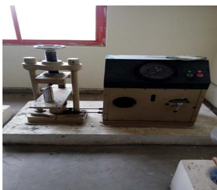
Figure 6: Flexural testing machine. Depicts the flexural testing machine using which the flexural strength of the beam samples are tested. It uses a two point load test system on the beam.
