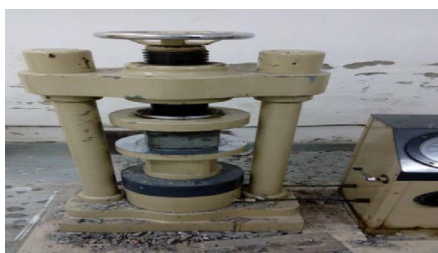
Figure 5: Compression testing machine.
