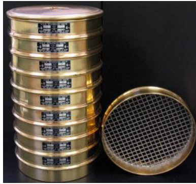
Figure 1: Sieve analysis of fine aggregates.
