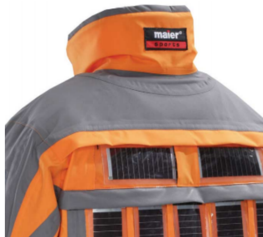
Figure 21: An example of a jacket with integrated solar cells. This model was designed to power an mp3 player.
