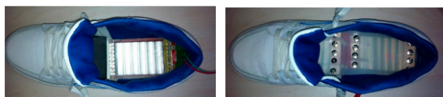
Figure 16: Two different piezoelectric-operating energy harvester prototypes created during research conducted at Tsinghua University.
