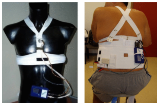
Figure 12: The BIOTEX system with sweat-analyzing sensors in a waistband (right) and a chest band (left) which collects ECG, respiration, and pulse oximetry information.
