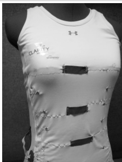
Figure 11: Piezoresistive sensors implanted in a shirt for monitoring respiratory conditions.
