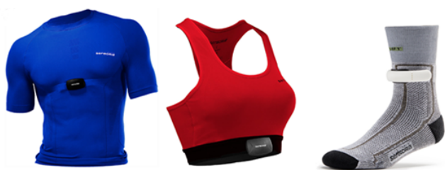
Figure 9: From left to right: sensoria men are smart t-shirt, sports bra, and socks. The heart rate monitors are placed near the center of the wearer's torso, and the anklet can be seen magnetically attached to the sock.
