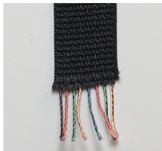
Figure 17: Ohamtex has developed textile cabling that does not affect the feel or properties of textiles.
