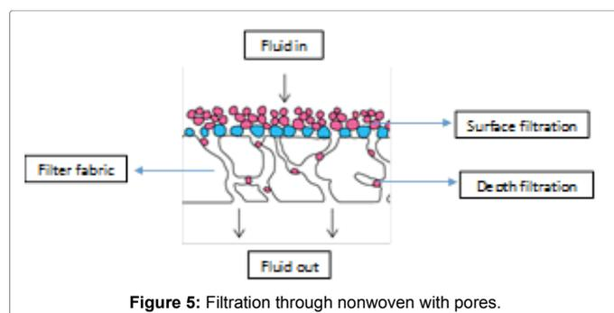
Figure 5: Filtration through nonwoven with pores.
