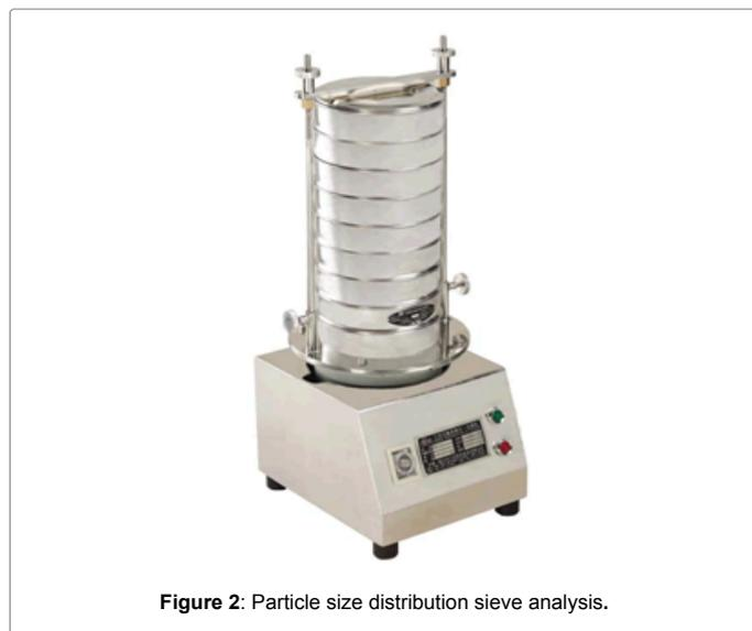
**Figure 2:** Particle size distribution sieve analysis.
