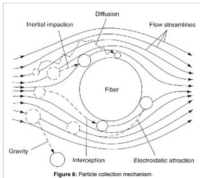
Figure 6: Particle collection mechanism.
