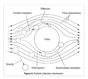
**d**) **Electrostatic deposition:** Submicron particles are difficult to capture even with combination of mechanical methods. It is well known that strong electrostatic forces of fibres attract the particles. Therefore, fibers may be given permanent electrical charges to attract small or medium sized particles.
