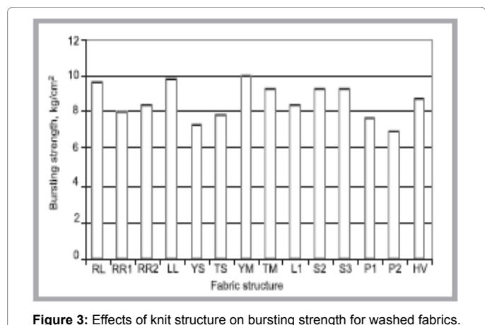
**Figure 3:** Effects of knit structure on bursting strength for washed fabrics.
