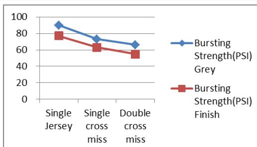
**Figure 7:** Bursting strength of cross miss fabrics.
