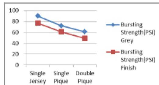
**Figure 5:** Bursting strength of pique fabrics.
