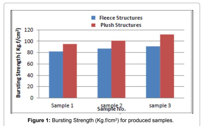
Figure 1: Bursting Strength (Kg.f/cm<sup>2</sup>) for produced samples.
