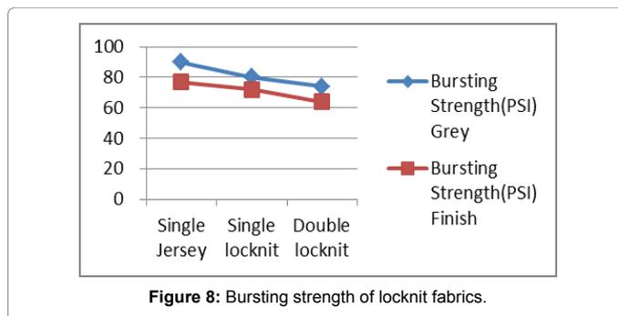
Figure 8: Bursting strength of locknit fabrics.
