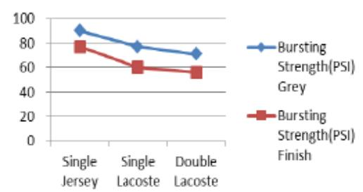
**Figure 6:** Bursting strength of lacoste fabrics.
