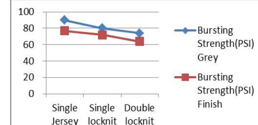
**Figure 8:** Bursting strength of locknit fabrics.
