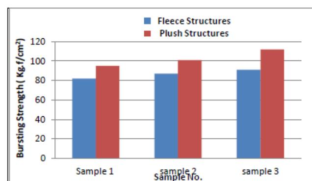
Figure 1: Bursting Strength (Kg.f/cm<sup>2</sup>) for produced samples.
