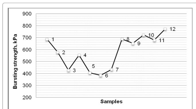
Figure 2: Bursting strength of gray fabrics according to the number and location of tuck stitches.
