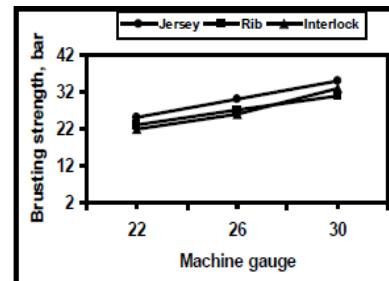
**Figure 4:** Effect of knitting machine gauge on knitted fabric Bursting strength for different knit structures.
