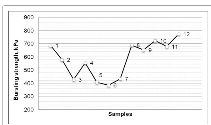
**Figure 2:** Bursting strength of gray fabrics according to the number and location of tuck stitches.
