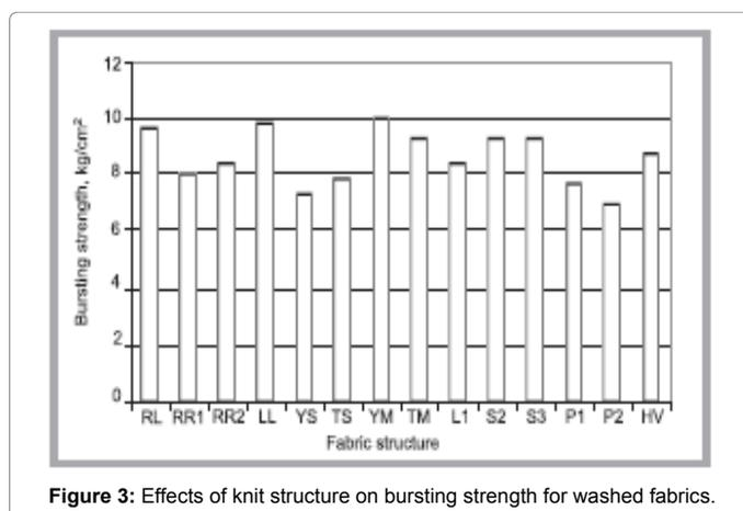
Figure 3: Effects of knit structure on bursting strength for washed fabrics.
