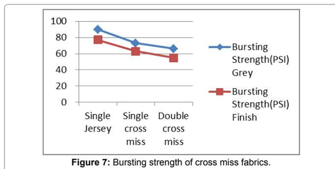
Figure 7: Bursting strength of cross miss fabrics.
