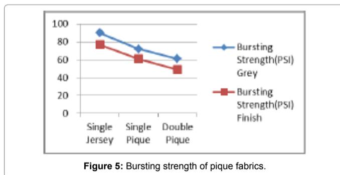
Figure 5: Bursting strength of pique fabrics.
