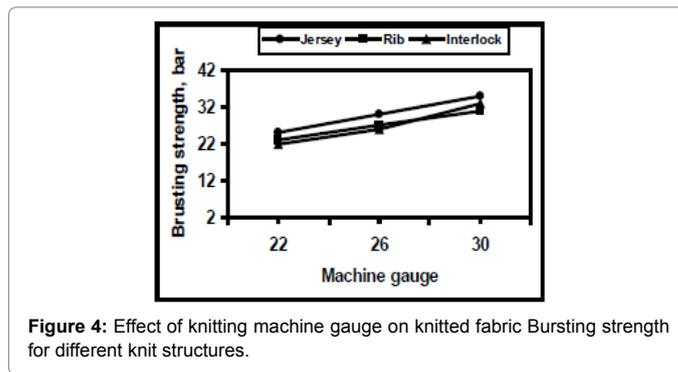
Figure 4: Effect of knitting machine gauge on knitted fabric Bursting strength for different knit structures.
