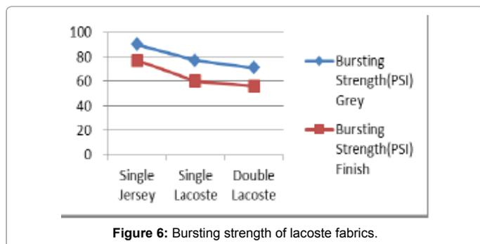
Figure 6: Bursting strength of lacoste fabrics.
