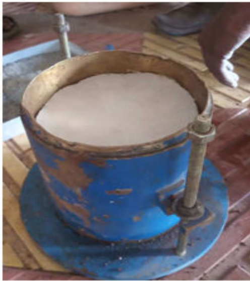
Figure 4. Making of CGT layer in CBR mould by placing geotextile over stone dust.
