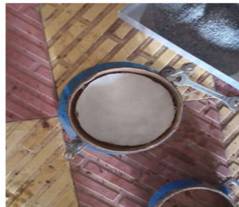
Figure 2. Making of CGT layer in CBR mould by placing geotextile.
