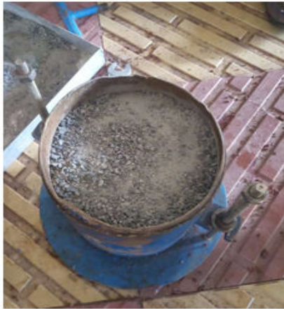
Figure 3. Making of CGT layer in CBR mould by laying of stone dust layer.
