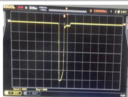
Figure 17: Output voltage measured on oscilloscope across a capacitive divider of 1/100.
