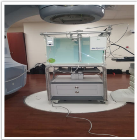
Figure 1a: Showing the set-up of phantom and ion chambers
