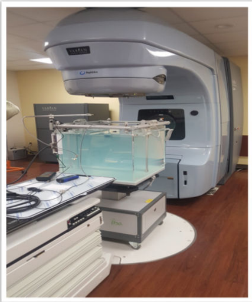
Figure 1b: Showing set-up of phantom and ion chambers.
