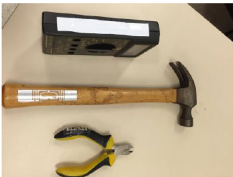
Figure 12: Tools with RFID tags (Barbosa, et al 2016) [41].
