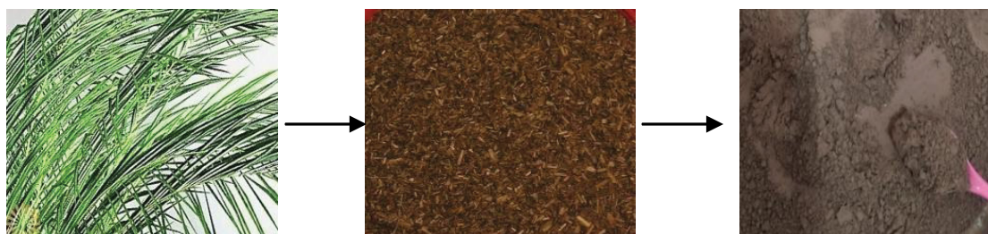
Figure 1. Raw palm leaves, cut to small size and pre-carbonize at 280°C before being milled to a fine grain for 50 hours.
