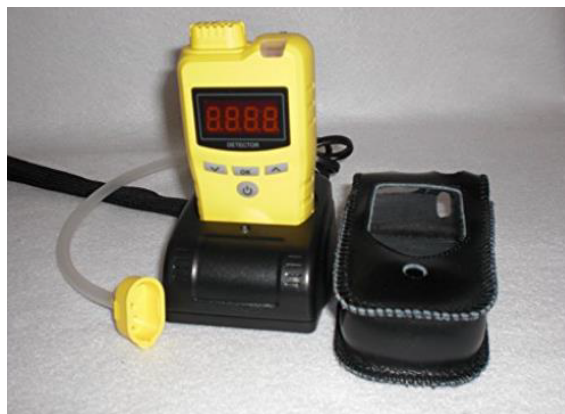
Figure 4: Essential to any clandestine laboratory producing BHO is the butane detection and alarm system. For sale on common internet sales websites the environmental monitoring of butane concentrations are used because of the high probability of explosions.
