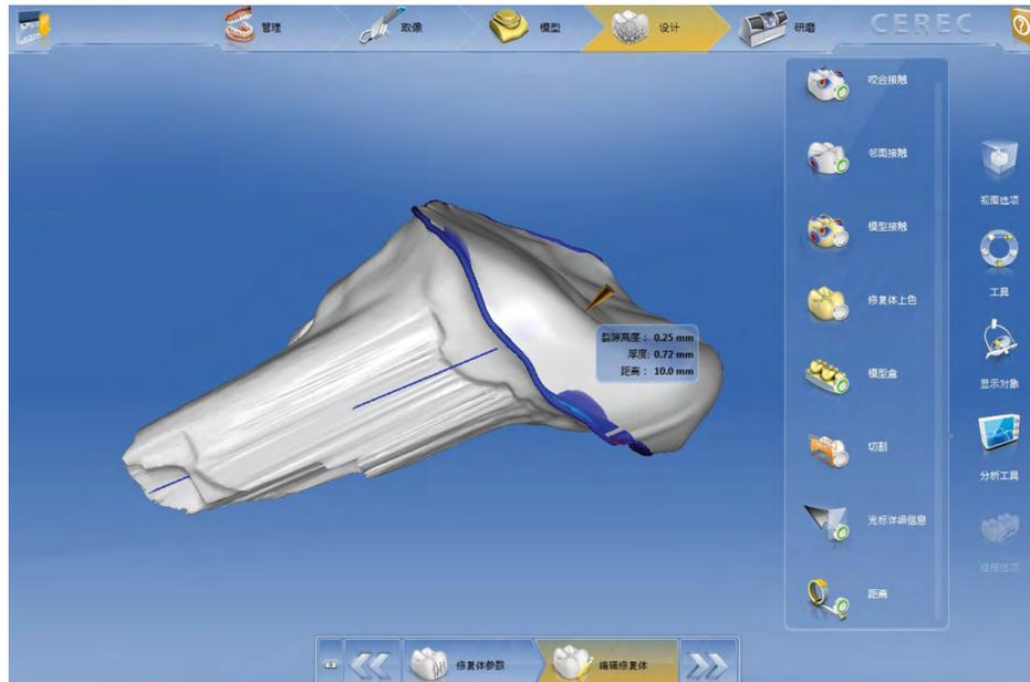
**Figure 4.** The height of post-core was 10 mm, less than the control of the CEREC intraoral 15 mm scanning depth.
