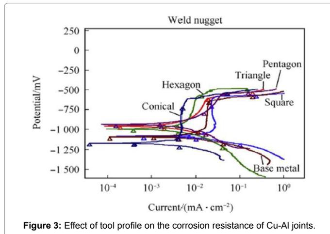
Figure 3: Effect of tool profile on the corrosion resistance of Cu-Al joints.
