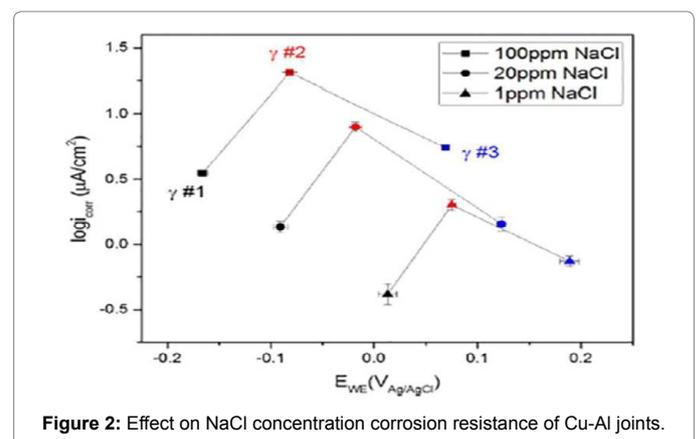
Figure 2: Effect on NaCl concentration corrosion resistance of Cu-Al joints.
