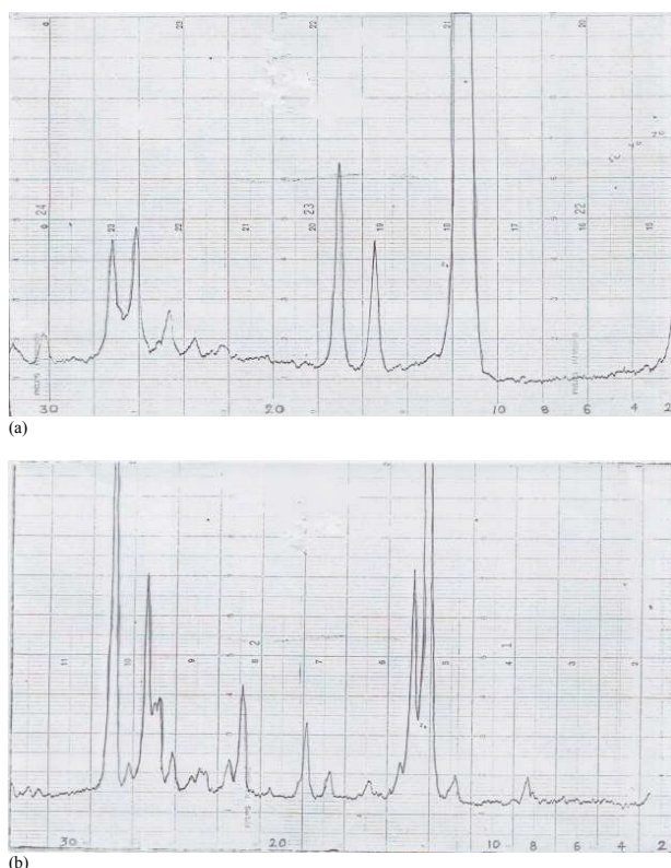
Figure 3: X-ray diffraction patterns of (a) Cu-Me and (b) VO-Me complexes.
