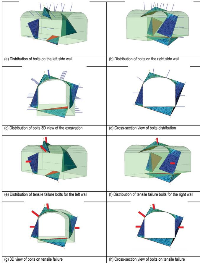
**Figure 9.** (a-d) Distribution of cable bolts installed at the spacing of 2.5 m by 2.5 m in plane and out of plane respectively, along the desired excavation and (e-h): Distribution of cable bolts that could fail through tensile failure mode along the simulated wedges in the excavation with 2.5 m by 2.5 m spacing.
