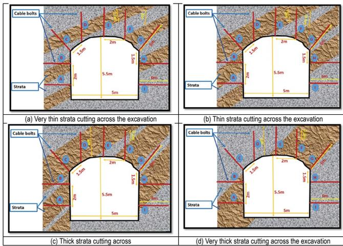
Figure 10. Simulated underground excavation with varying strata thickness.
