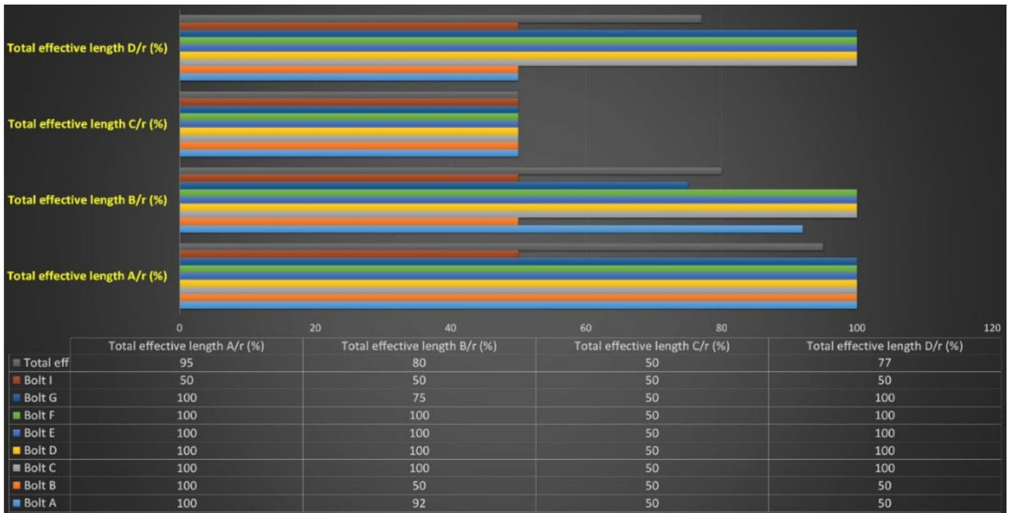
Figure 13. Calculated effective length of the bolts using the simulated examples in conditions of varying orientations of the strata.
