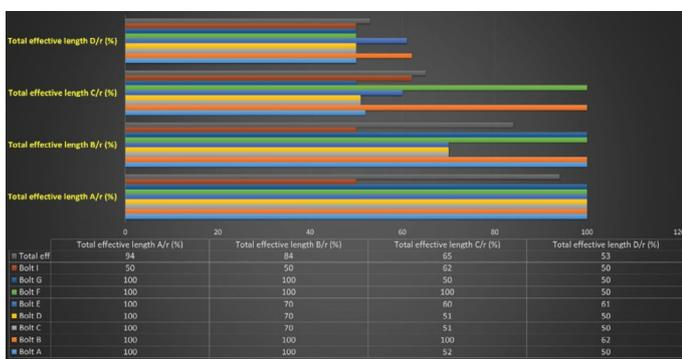
Figure 11. Calculated effective length of the bolts using the simulated examples in conditions of varying thickness of strata.
