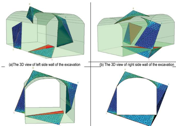
Figure 5. (a-d) Simulated FS of an excavation in a deep level environment, with three significant wedges denoted on the hanging wall and sidewall. Note that the footwall wedge is not of interest in this study.
