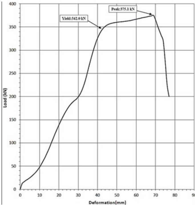
Figure 4. Third static loading test results of a Mechanical anchor (38 tons, 18 mm, and 6 strands).
