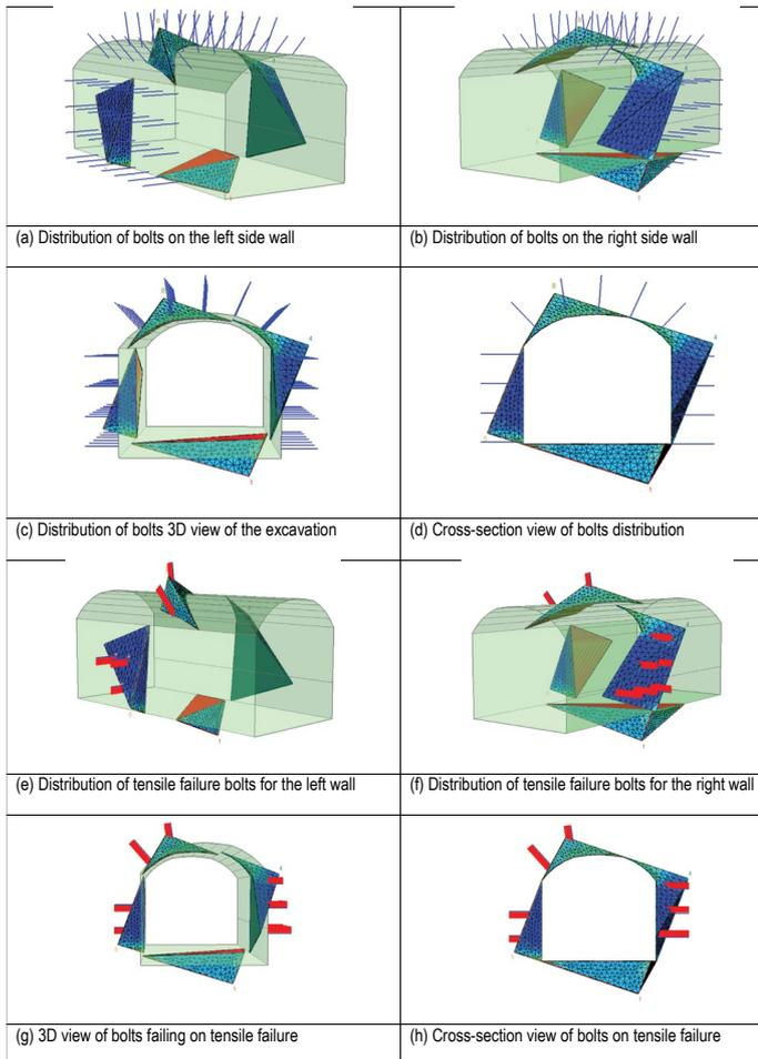
**Figure 7.** (a-d) Distribution of cable bolts installed at the spacing of 1.5 m by 1.5 m in plane and out of plane respectively, along the desired excavation and (e-h): Distribution of cable bolts that could fail through tensile failure mode along the simulated wedges in the excavation with 1.5 m by 1.5 m spacing.
