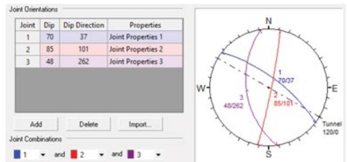
**Figure 2.** Stereonet of the simulated underground situation using Unwedge (Finite Element Method).
