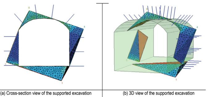
Figure 14. Simulated underground excavation with installed bolts using the normal to opening section.
