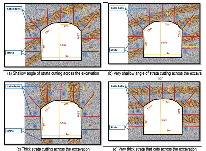
Figure 12. Simulated underground excavation with varying orientations.
