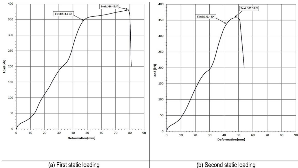
Figure 3. (a & b) Static loading tests results of a mechanical anchor (38 tons, 18 mm, and 6 strands).
