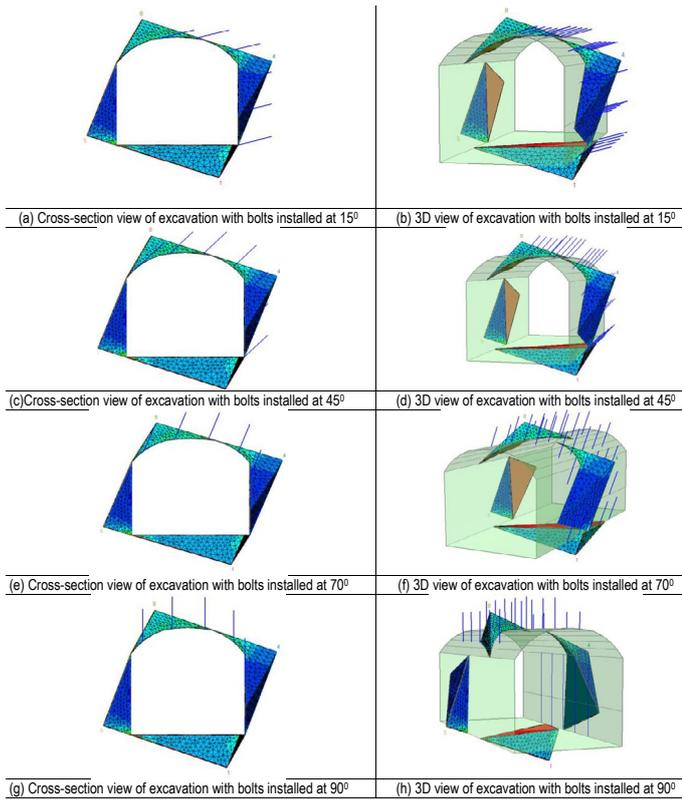
Figure 15. Simulated underground excavation with installed bolts using varying cable bolting.
