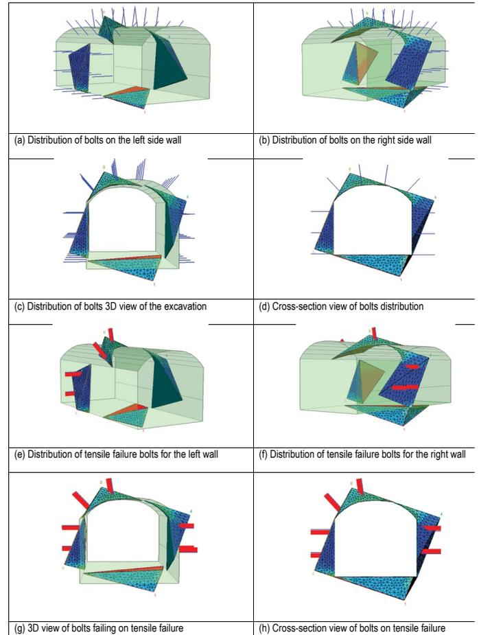
**Figure 8.** (a-d) Distribution of cable bolts installed at the spacing of 2 m by 2 m in plane and out of plane respectively, along the desired excavation and (e-h) Distribution of cable bolts that could fail through tensile failure mode along the simulated wedges in the excavation with 2 m by 2 m spacing.
