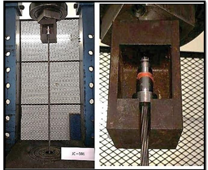
**Figure 1.** A mechanical anchor of 1.5 m, 18 mm diameter steel cable with 18 ton AMS barrel anchor assembly inserted into a testing machine before test with a barrel and wedge assembly on the top platen.
