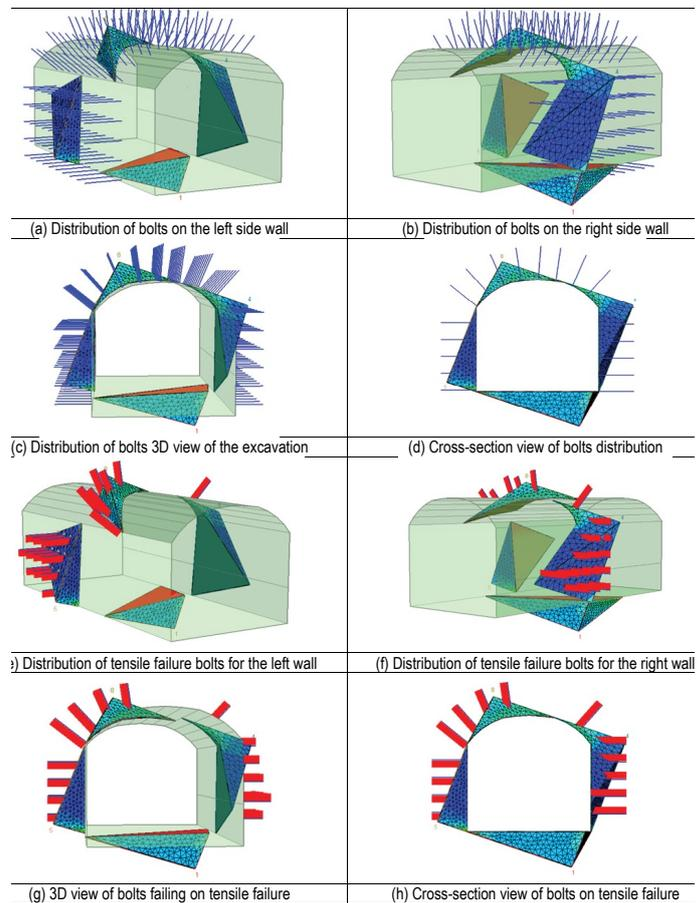
Figure 6. (a-d) Distribution of cable bolts installed at the spacing of 1 m by 1 m in plane and out of plane respectively, along the desired excavation and (e-h): Distribution of cable bolts that could fail through tensile failure mode along the simulated wedges in the excavation with 1 m by 1 m spacing.
