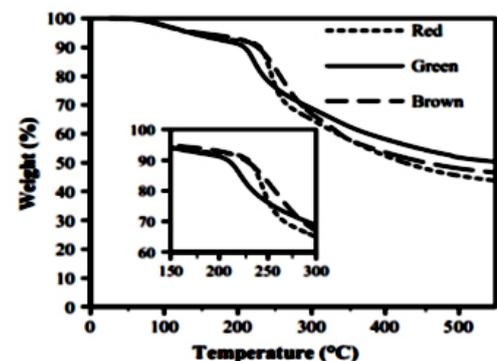
**Figure 4.** TGA (Thermogravimetric analysis) curve of red, green and brown algae flakes of 200-400 μm [73].
