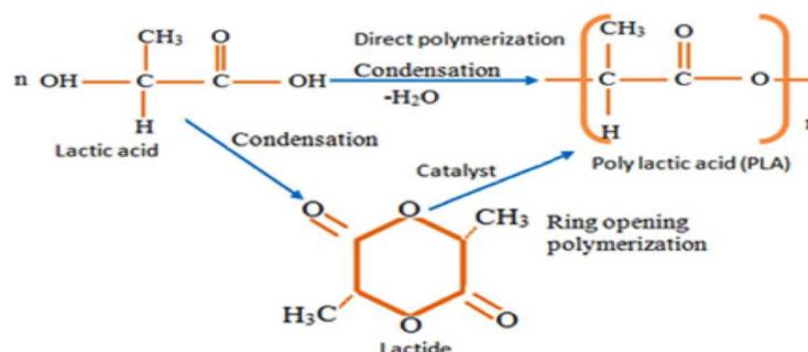
Figure 2. PLA polymerization [46].
