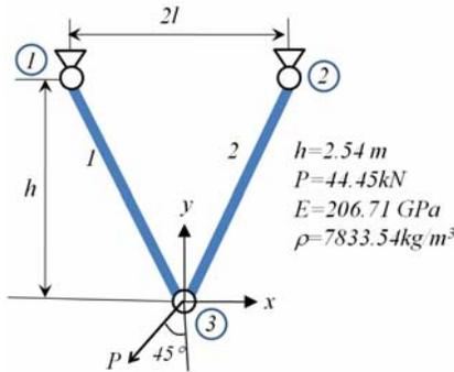
Fig. 1 Two-bar truss
