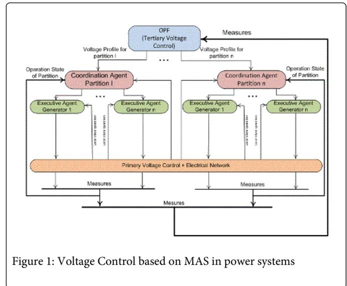
Figure 1: Voltage Control based on MAS in power systems
