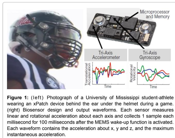
**Figure 1:** (left) Photograph of a University of Mississippi student-athlete wearing an xPatch device behind the ear under the helmet during a game. (right) Biosensor design and output waveforms. Each sensor measures linear and rotational acceleration about each axis and collects 1 sample each millisecond for 100 milliseconds after the MEMS wake-up function is activated. Each waveform contains the acceleration about x, y and z, and the maximum instantaneous acceleration.
