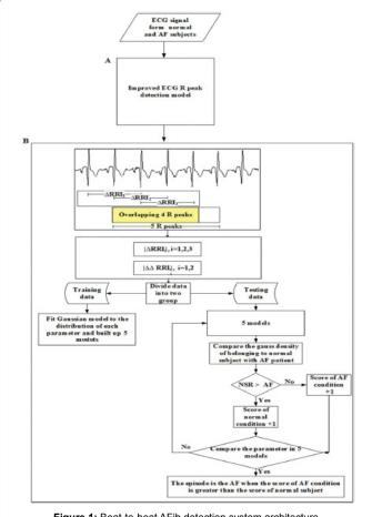
Figure 1: Beat-to-beat AFib detection system architecture.
