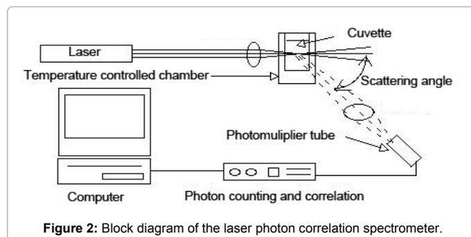
Figure 2: Block diagram of the laser photon correlation spectrometer.
