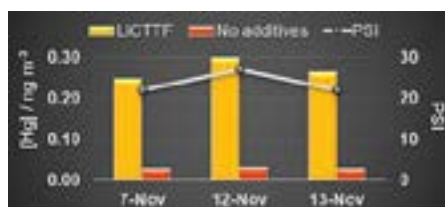
Figure 1: Detection of up to 10 times higher concentrations of mercury with addition of tetrathiafulvalene aids.
