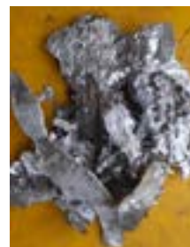
Figure 3. shown how carbon deposits on the surface of the molten alloyed
