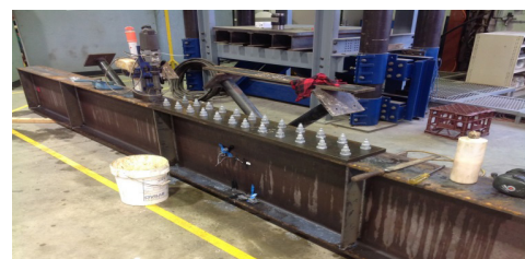
Figure-2: Retrofitted section for new 610UB113 equivalent girder.
