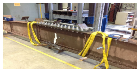
Figure-1: Retrofitted section for RMS 120-year-old girder.
