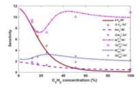
Simulated and measured sensor sensitivity versus the gas concentration. Here the sensitivity was calculated considering a typical single statistic feature (peak amplitude (A) and the mean (m1)) and considering some of our tailored functions based on the combination of two statistics features (fm and fA).
